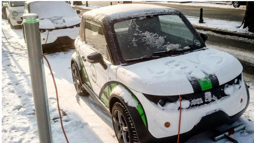
*Your EV battery doesn't like extreme cold weather any more than you do, but plugging in allows the EV thermal management systems to help keep the battery comfortable.*
